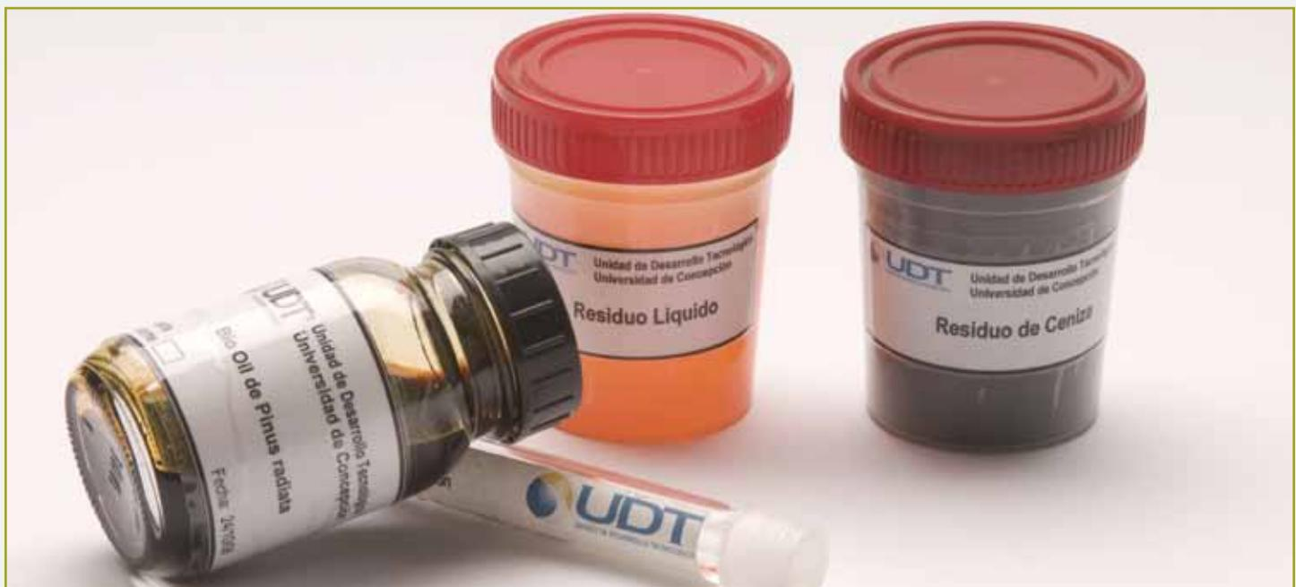
is an available technology that turns low-energy-density solid waste in a liquid fuel of higher calorific value, easy to transport, store and distribute, decoupling the production and use of energy. The liquid or bio-oil is a new fuel with different characteristics and incompatible with fossil fuels, which has prevented, so far, its market introduction.
