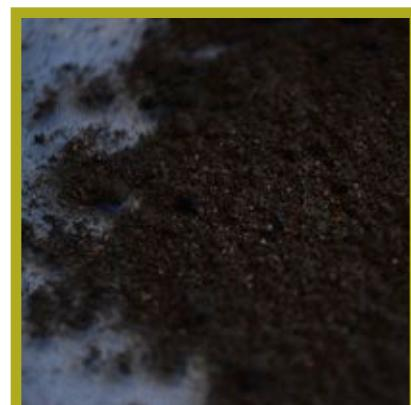
It is thus necessary to modify the properties of biomass through thermochemical processing that produces an energetically densified biofuel, whose physico-chemical properties (high calorific value, low moisture content, homogeneity and hydrophobicity) make it more competitive than coal.
